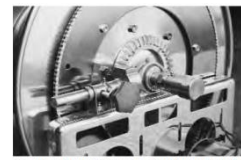
Optional Auxiliary Rewind (Ring and chain rewind unit with removable crank handle)
